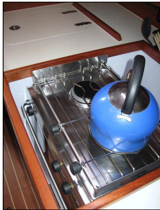
Stove with gimbal, safety bar and pot clamps.
