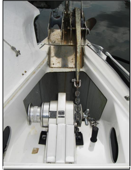
Anchor windlass and ground tackle
